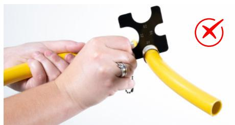
If the template does not fit, the crimping is outside the pressing tolerance. In this case, it is necessary to calibrate the tool according to the manual.
