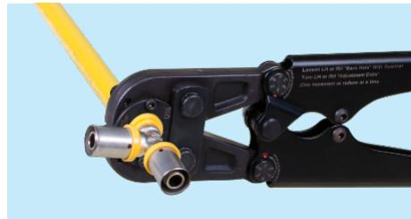
3. Place the tool on the yellow part of the fitting and perform the crimping.
