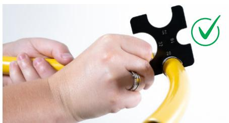
Insert the pipe into the opening of the template corresponding to its diameter. If the fit is correct, the crimping is correct. However, if the pipe does not fit or is loose, the crimping is incorrect.
