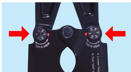
1. The tool has two adjustment pins, as indicated in the image with red arrows. To make the adjustments, it is necessary to adjust one pin at a time.
