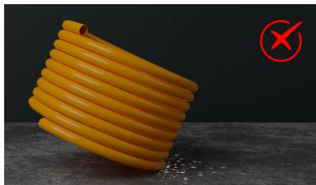
During transportation and storage, the pipes should be placed on a flat, dry, non-abrasive surface, away from sharp objects, and at an ambient temperature below 60°C. Also, the pipes should not be dragged on the floor or subject to any friction.
