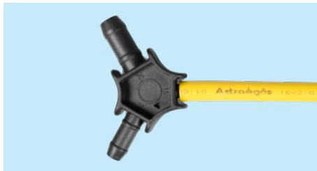
1. Each end of the calibrator indicates a different diameter. Insert the pipe into the corresponding size end and rotate the calibrator 3 to 4 times.
