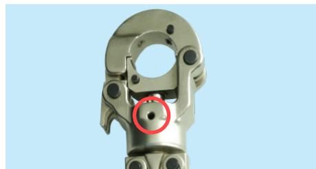
1. Loosen the screw (location indicated in the image) with the adjustment key.
