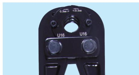
**1.** Choose the correct crimping insert (the appropriate insert should have the same diameter as the external size of the pipe to be crimped).
