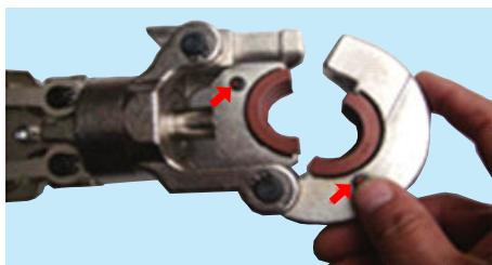
3. Press the pins to position the inserts into the head of the tool.
