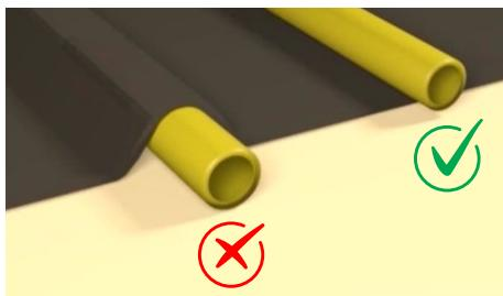
Do not cover the pipe with insulating or waterproofing blankets to avoid overheating.
