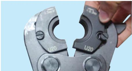
**1.** Select the correct crimping insert (the appropriate insert for crimping should have the same diameter as the external size of the pipe to be crimped).
