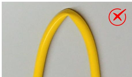
Do not bend the pipe. If this happens, the material cannot be used as the damage is permanent.
