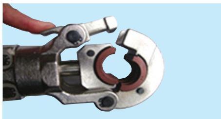
2. Open the tool handles and release the safety lock.
